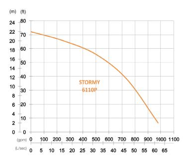
Shaft Speed: 1450 rpm Outlet: 150mm, 6in
